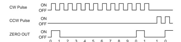
※ ZERO OUT means the initial status of motor excitation (STEP 0), it outputs per 7.2° of rotation in Full Step. (It outputs 50times per 1 rotation of motor.)
