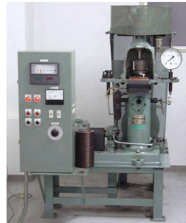
Photo B-14 : SOTA-4-Ball wear test machine
