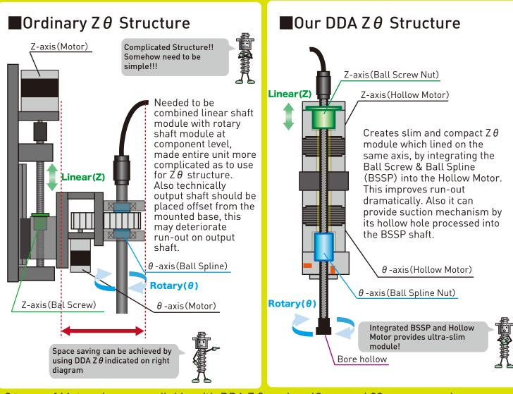
2 types of Motor size are available with DDA Z  $\theta$  series, 42mm and 28mm squared. Travel length and the Load Capacity can be selected with Motor size.
