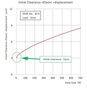
To be more accurate, it is necessary to add Elongation by heat generation or deformation by torsion. But they can be disregarded in case of Miniature Ball Screws.
