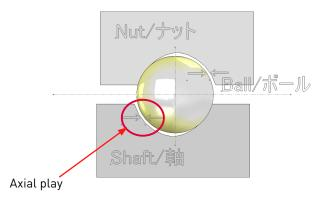
If Ball Screws receive Axial load, groove of Shaft and Nut contact to Ball, after that the Elastic displacement will appear on the contact surface. Total of initial clearance (Axial play) and Elastic displacement becomes Backlash (see figure below).
