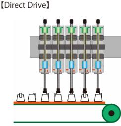
Suitable for use as multi-connected unit, because of its slim body which is mounted all the components, such as Motor and drive shaft on the same axis. include all the components such as Motor and working shafts lined and mounted within the same level.
