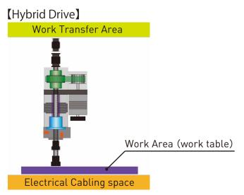
Suitable for use in the limited area in height, because of its compactness of Actuator body length.
