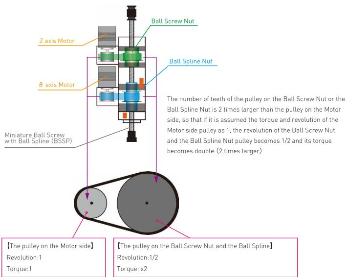
Torque is increased twice as much by changing the size of the pulley!
